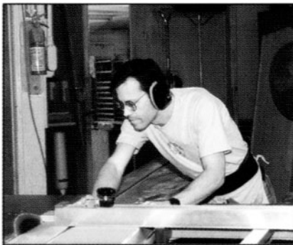
Bernie Becker, co-owner, operates the shop's Holzma sliding table saw. Becker often adds lifts, retractable doors, or pull-outs to customize products.
